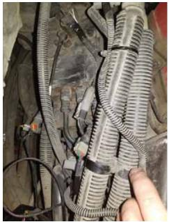
**6)** Connect the red wire with a ring terminal to a constant 12 volt source. Connect the black wire with a ring terminal to a good engine ground. Wiring can be routed over the engine to the Alternator. Note: For RV's, power and ground needs to be connected to the engine, not the house battery system.
