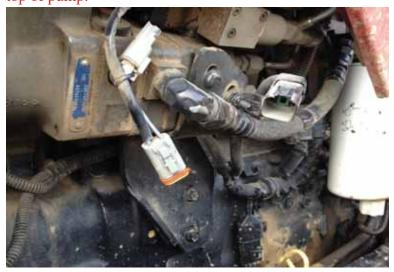
3) Connect the female injection control valve connector from the module into the stock male connector.
