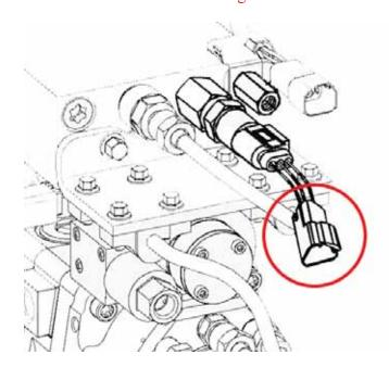
**5)** Plug the female fuel pressure connector into the factory male connector. Plug the male fuel pressure connector into the stock female connector.
