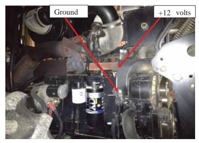
7) Mount the module in a safe location using the supplied wire ties. Secure the module away from any excessive heat and
