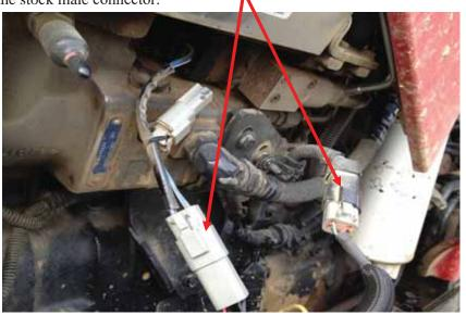
**4)** locate the fuel pressure sensor as shown in the diagram. and unplug.
