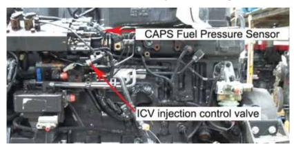
2) Connect the male injection control valve connector from the module into the stock female connector.
