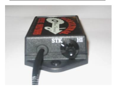
The module above is shown in the stock position. Stock is all the way to the left (counter clockwise). Move the rotary switch to the Middle for the Low Position and to far right for the High Position
