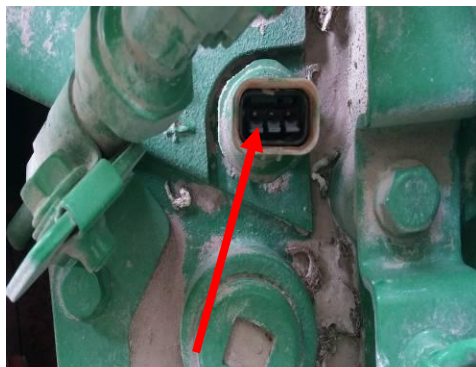
Plastic keyed terminal lock, stuck inside MAP Sensor
